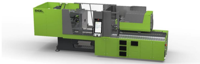
Image 1: More mould space with a smaller footprint, the new electric ENGEL victory electric 220 with 2,200 kN clamping force enables compact production through its tie-bar-less design and shortened machine length.
