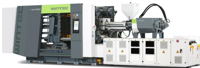
Image 6: The WINTEC t-win 5500 two-platen injection moulding machine with integrated viper 40 robot will produce transparent PP crates weighing 232 grams, with a cycle time of 11-12 seconds, demonstrating high-output production with reliable automation and competitive unit costs.
