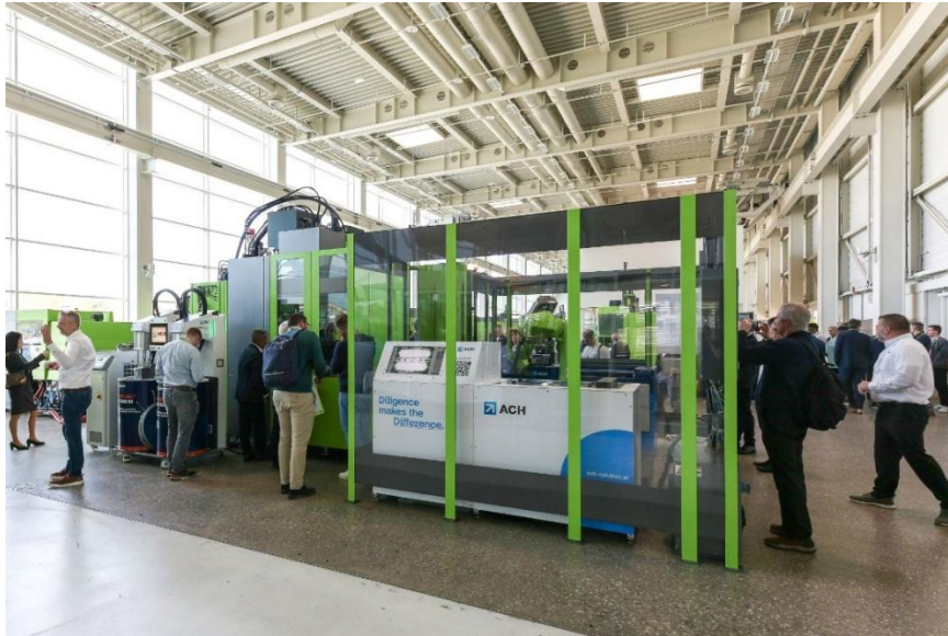
Image 2: In the production of GDL films for fuel cells, the vertical ENGEL insert 150 shows how sensitive film components can be overmoulded with LSR precisely, reliably and cost-efficiently with high output.
