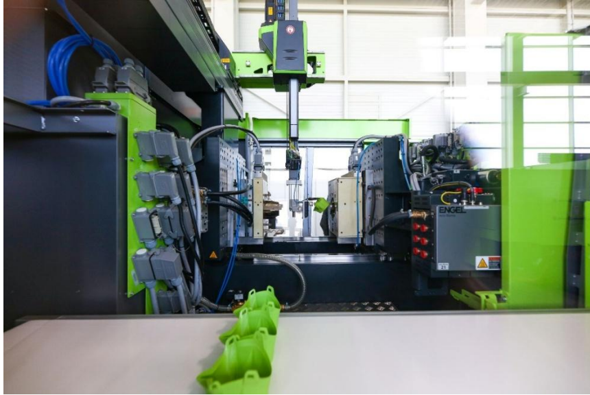
image 3: The tie-bar-less ENGEL e-victory 160 offers greater flexibility in mould design with its large free mould space and large platens. This can help to select a smaller machine size and reduce investment costs.
